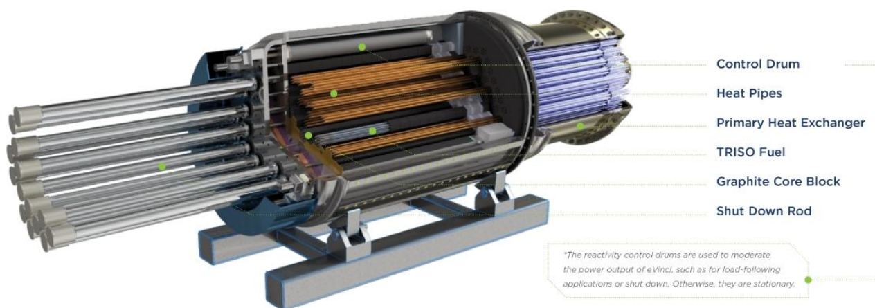
Figure 8: Schematic image of the eVinci core, taken from [119].
