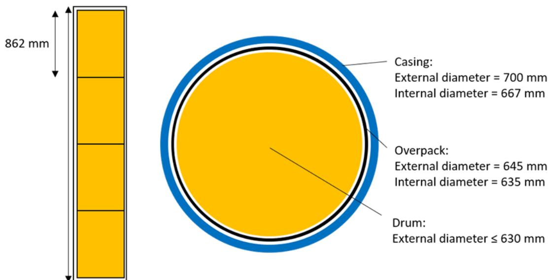
Figure 6: Sketched overpack for 200-liter drums, shown from the side (left) and axially (right).
