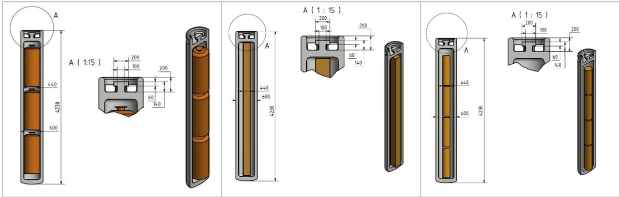
Figure 2: Canister with reprocessing waste (left), SNF (Krško NPP, middle), and Danish waste (right). Figure made by BGE-TEC.
