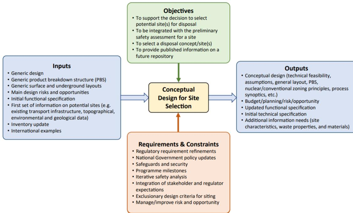
Figure 5: Conceptual design for site selection: objectives, inputs, constraints, requirements, and outputs [31].
