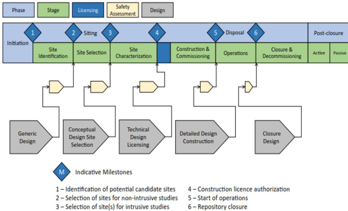
Figure 3: Design, siting, and licensing of radioactive waste repositories [31].
