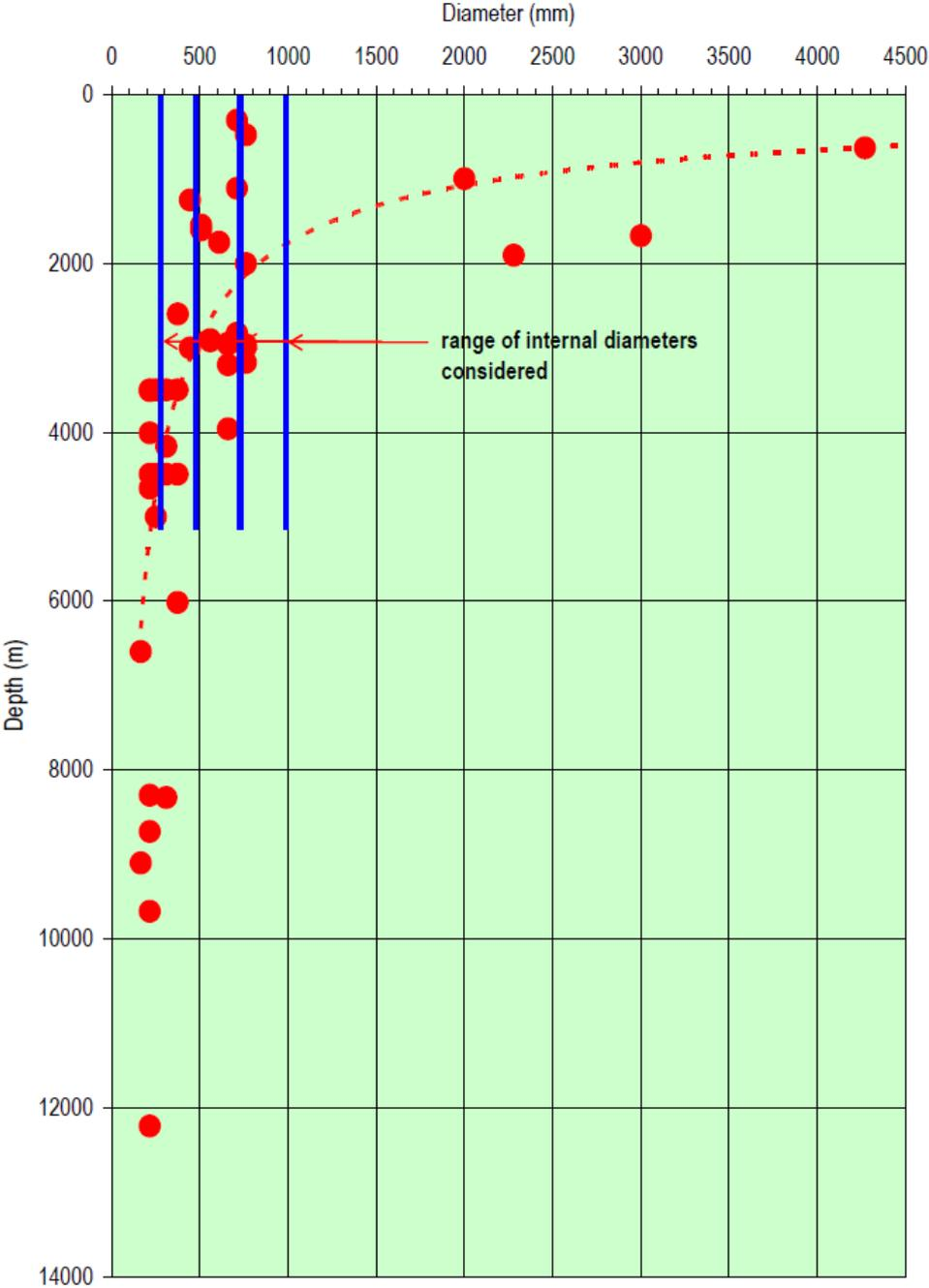
Figure 1: Depth and diameter of boreholes drilled until 2008 [12].
