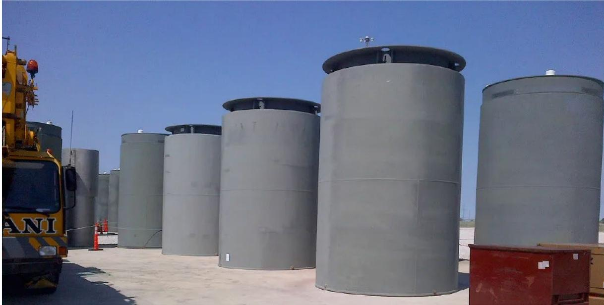
Figure 8: HI-SAFE containers. Photo: Holtec International (<https://holtecinternational.com/products-and-services/nuclear-fuel-and-waste-management/dry-cask-and-storage-transport/hi-safe/>).
