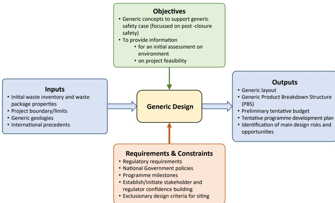
Figure 4: Generic design: objectives, inputs, constraints, requirements, and outputs [31].
